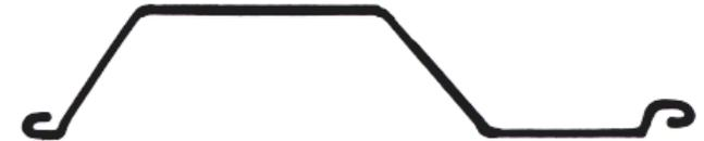
**Arch shaped and lightweight "gauge" sheets (A)** used for shallower wall construction.
